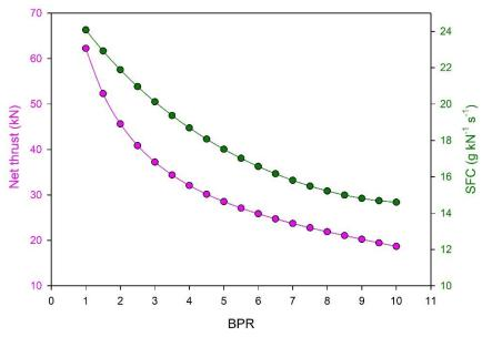
Figure 9. Net thrust and SFC variation relative to BPR
