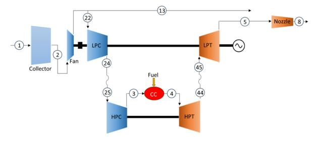
Thermodynamic schematic of the modelled engine
