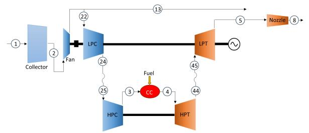
Figure 1. Thermodynamic schematic of the modeled engine
