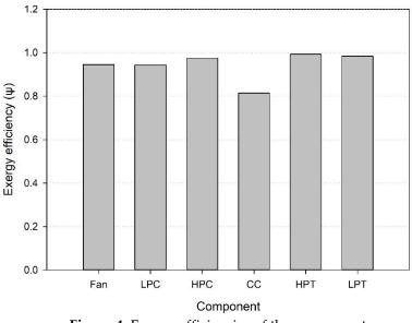
Figure 4. Exergy efficiencies of the components
