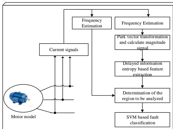
Figure 3. Information entropy-based stator fault diagnosis
