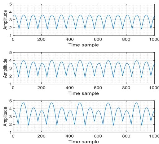
**Figure 6.** Feature signals for healthy and two fault states (a) Solid, 5% and 10% of fault resistance altered fault.
