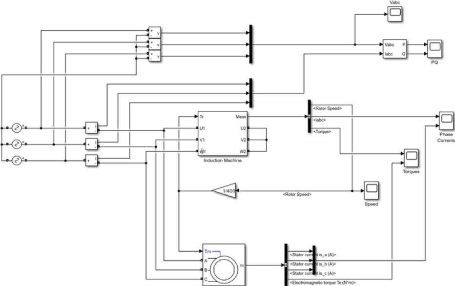
Figure 1. 500W Induction motor model obtained using the voltage approach behind the reactance
