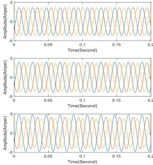
**Figure 5.** Current signals for solid and two fault states (a) Solid, 5% and 10% of fault resistance altered fault
