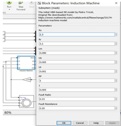
Figure 2. Fault rate and fault resistance change screen
