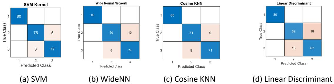
**Figure 8.** Fault classification with different machine learning approaches.
