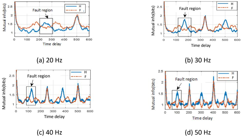
**Figure 7.** Mutual information of healthy and faulty conditions for different operating frequencies
