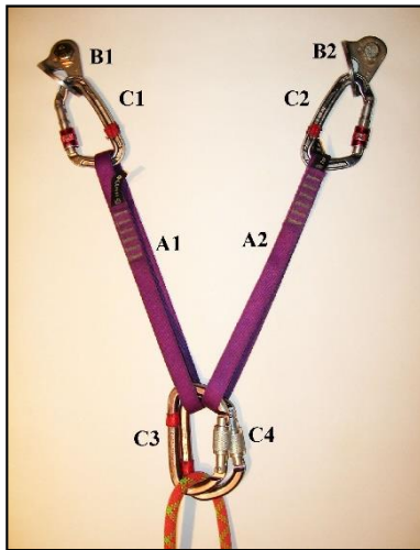
Figure 3. Two slings and four locking carabiners employed to set up a truly redundant but non-adjusting anchor system. Rope attached to reversed D carabiners.
