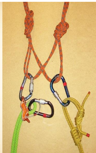
Figure 10. Quad multi-pitch setup, with system elements conveniently spaced apart. The belay is on the left and the belayer's Purcell Prusik leash (PAS) is on the right.
