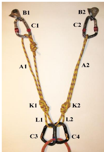
Figure 8. Quad with separated carabiners using a single cord. Rope attached to separated HMS carabiners and cord segments isolated with two Overhand Loops.
