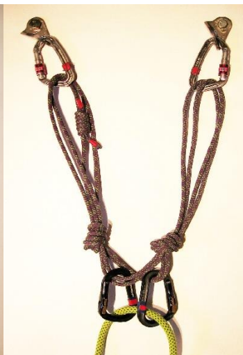
Figure 9. Quad with separated carabiners using a double cord. Rope attached to separated HMS carabiners and cord segments isolated with two multi-strand Overhand Loops. (Figure 8 labels apply to this image as well.)
