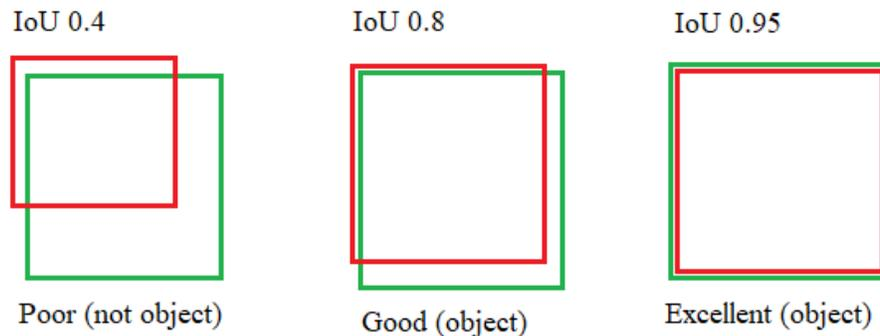
FIGURE 5. An example of IoU for different bounding boxes.
