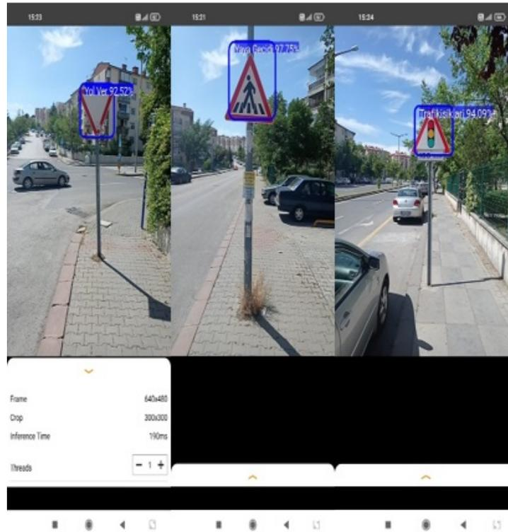
FIGURE 8. Detected Traffic Sign in the mobile app.
