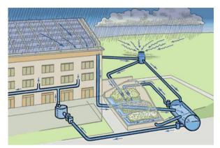
**Figure 9.** Rainwater Harvesting System at Yale University: Stormwater from the roof and the ground collects in a tank at upper right, which empties into a pond, where it is cleansed and diverted into larger harvesting tank. The water in harvesting tank is pumped to another tank for use inside and back into the pond.
