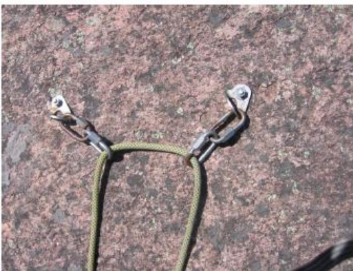
Figure 3. Expansion bolts with paired quick links.
