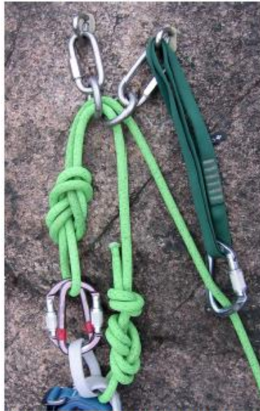
Figure 5. Lowering – Loop-Feed Method: For simplicity, the personal anchoring system (PAS) is omitted in the photograph. The green sling to the right represents either a quick draw for leaders, or a top-rope setup. The loop is fed through the anchor, a Figure Eight Loop is tied and clipped to the harness, and the original harness tie-in is removed.
