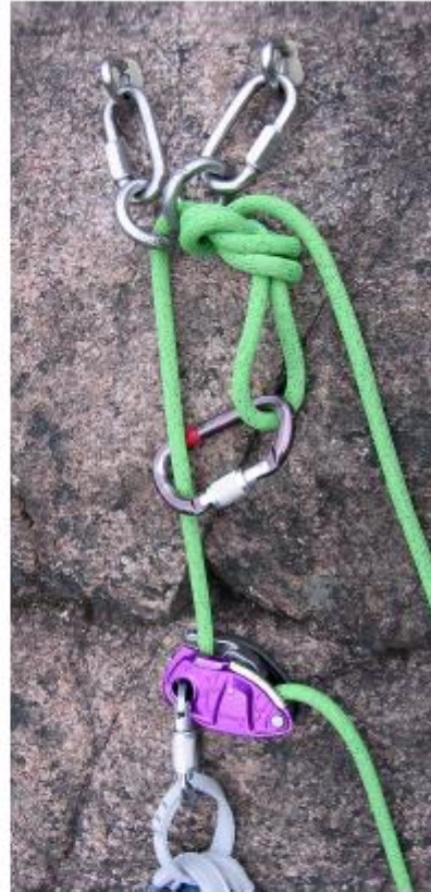
Figure 8. Rappelling – Single-Line Rope-Retrieval Method: The rope was fed through the closed anchor system until the halfway point reached the anchors. The load-bearing side of the rope is secured with a Figure Eight Loop and a locking carabiner. An assisted-braking device secures the harness to the load-bearing side of the rope.
