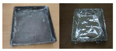
Fig. 1 The die which is used for creating test samples
