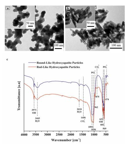
*Figure 1.* Nanoparticle characterization. *TEM images of different shapes of hydroxyapatite particles round-like (a) and rod-like (b). FT-IR spectra of round-like and rod-like hydroxyapatite particles (c)*
