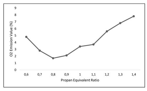
Figure 2. O<sub>2</sub> emission value at different propane equivalent ratio
