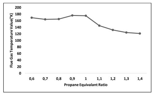
**Figure 7.** Flue gas temperature values at different propane equivalent ratios
