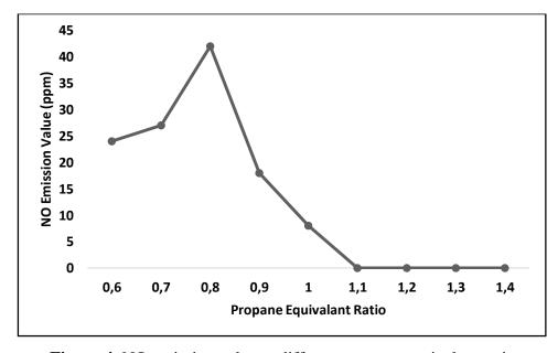
Figure 4. NO emission value at different propane equivalent ratio
