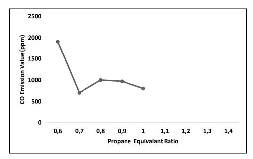
**Figure 5.** CO emission value at different propane equivalent ratio
